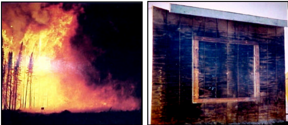
Figure 4 — (left) the experimental crown fire with flame heights about 20 meters; (right) wall section after the crown fire exposure--scorch but no ignition. Note the lack of scorch under the eave due to "shading" of the flame radiation.
